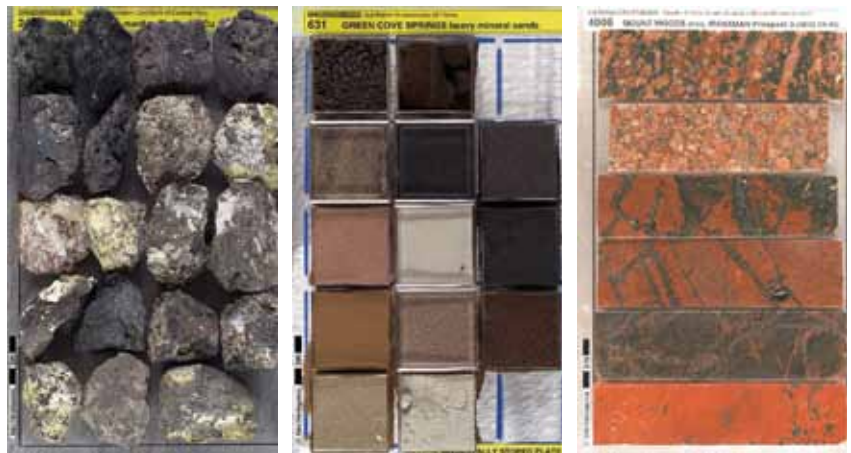
Figure 1. Variety of Lithotheque plates (the 7 x 11 inches plate size is constant). LEFT: standard layout of 20 solid samples, Colquijirca Pb-Zn-Ag. CENTER: powdery or friable samples held in plastic “jewel boxes”. RIGHT: oversize drill core slabs.
