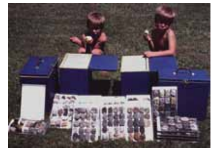
Figure 8. Portable Lithotheque of Tasmanian (Australia) deposits and geology to provide physically testable record and a standard for description and interpretation.
